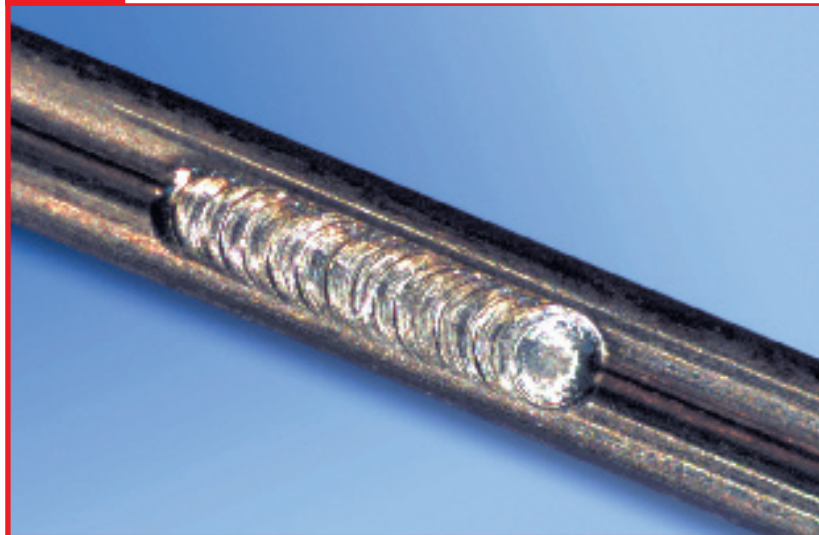
Figure 1: Fine stainless steel wires of 0.25 mm diameter joined by laser welding.
