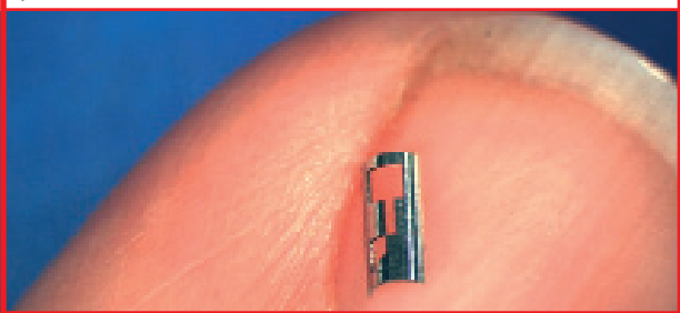
Figure 1: Small components with dimensions measured in \mu\text{m} rather than mm can be laser cut from tube or sheet.
