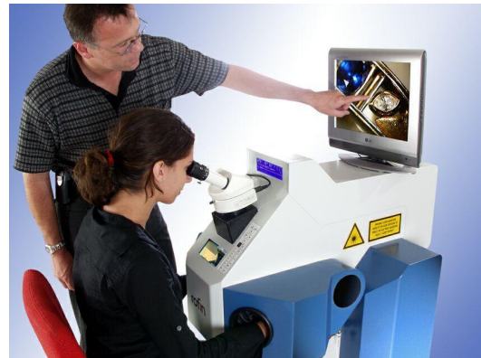
The StarWeld Performance Laser Microwelder specifically designed for spot or seam welding of different metals or metal combinations
