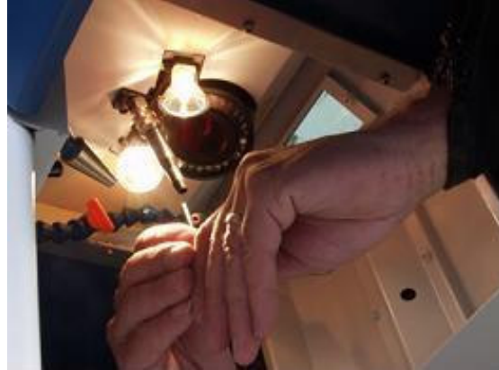
Parts to be welded are held in position by hand – the most flexible and versatile welding results are possible
