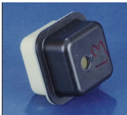
FIGURE 3: Laser welded test box
